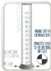
Figure 2 Turbidity Test
