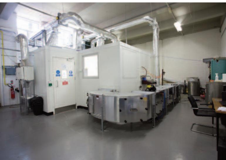
Our large, temperature & humidity controlled AHAM type environmental chamber, attached to a test duct rig system (ASHRAE 52.2 modified) used to simulate real-world environments.
