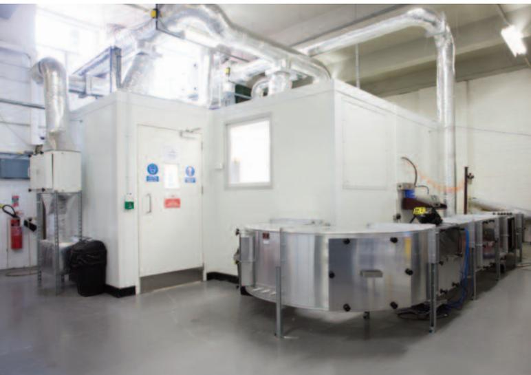
28.5m<sup>3</sup> AHAM type chamber, with controlled temperature, humidity and air change, used to simulate real-world environments
